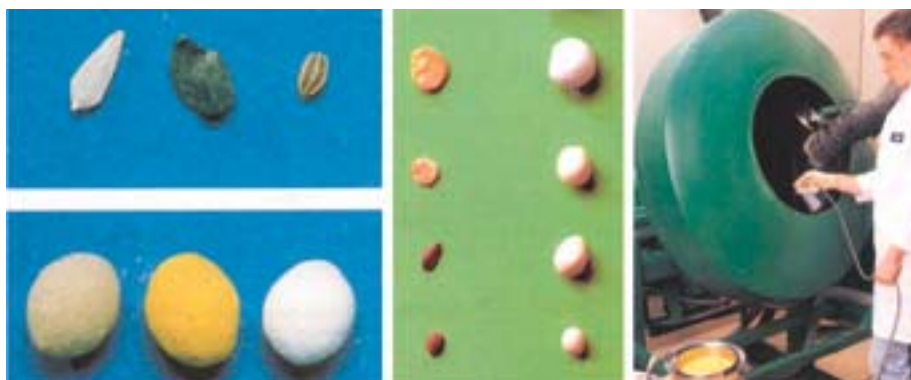
Figure 6. Pelletizing machine (right) vegetable seeds pelletized and colored. From left: Raw (top) and pelletized (bottom) seeds of lettuce, onion, and pepper, tomato, lettuce, and carrot seeds, respectively.
